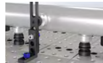
Vertical application using Locating Post + V-Block Spacer
