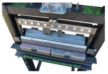
The side stop has notch marks laser cut on the top surface. Align the back stop with the center of these notches for quick repeatable bending. The first notch is 2" away from the center of the top die, the 2<sup>rd</sup> notch is 3" away, the 3<sup>rd</sup> notch is 4" away and so on. If using the HD press brake kit the first notch is 3" away from the first notch and the 2<sup>nd</sup> notch is 4" away and so on.
