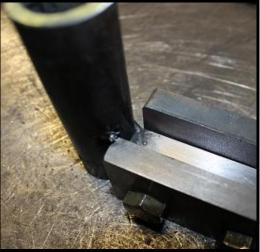
Once you have tacked the guide tube in a couple different locations, double check that the top die assembly will freely slide on the vertical guide tubes welded in step 1, adjust as necessary then fully weld both sides of the guide tubes. Take time to protect the machined area where the finger dies slide into, as welding spatter will easily stick to the clean machined surface if left exposed.
