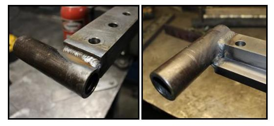
Depending upon the thickness of your weld it may be necessary to bevel the edge of the ½" thich threaded beam clamp to ensure it will sit flush.
