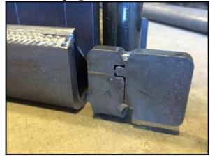
Using your shop press or a large hammer, press down on the  $\sim$ 7" long solid rod so the shaft is pressed half way through the bottom plate, note this will be a tight fit. From the bottom side, tack the rod into position,. Repeat this procedure on the other side.
